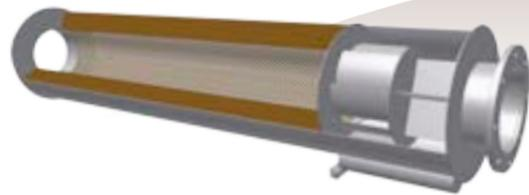
The noise is absorbed by specific acoustical fibre inside the silencer. The Absorption Type silencer is most effective in the middle and high frequency range.
