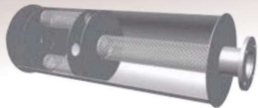
The noise is reduced by creating a gas flow through separate chambers in the silencer. The Reflection Type silencer is most effective in lower and middle frequency range.
